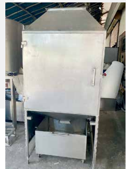
Gas Dust Burnout Furnace
